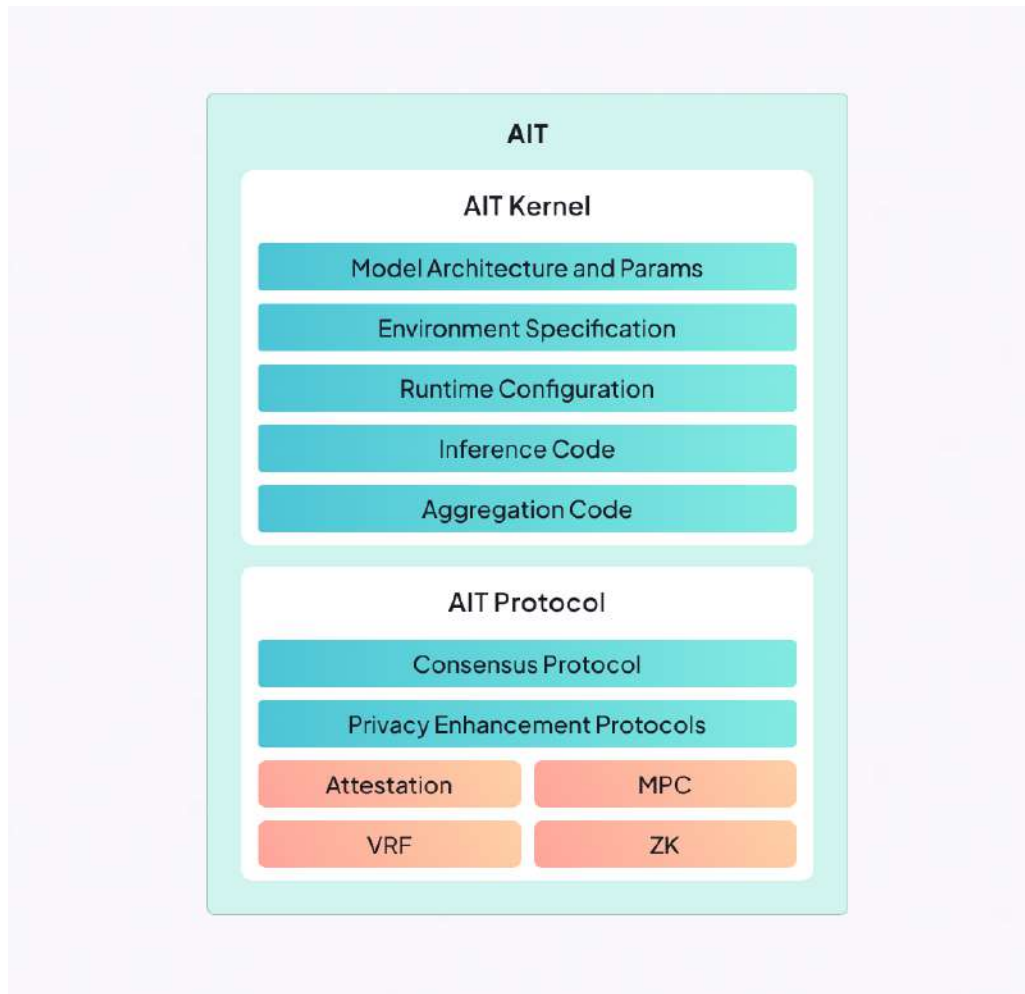
Figure 2.2: AIT Architecture. The AIT contains two core components: the AIT Kernel and the AIT Protocol. The kernel is stored on chain. Its primary purpose is ensuring that the query inference is carried out in a consistent way in the committee of nodes. The AIT Kernel contains specific information related to model inference, including model architecture and parameters, environment specifications, runtime configuration, and inference and aggregation code. Together this makes up the AIT Configuration File, a file functionally similar to a Dockerfile that details the dependencies, libraries, and runtime needed to run the model to ensure identical execution environment. The AIT Protocol's primary purpose is to facilitate communication among the nodes (mostly for security and privacy guarantee) and is packaged in software provided by us. The AIT Protocol includes the consensus protocol and privacy enhancement protocols, including Nesa's security mechanisms.
